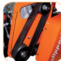
Pulleys with removable hub and Poly V belts.
