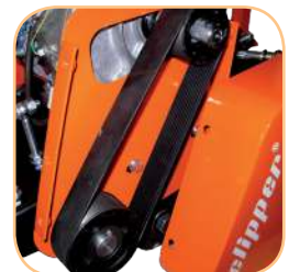
Pulleys with removable hub and Poly V belts.
