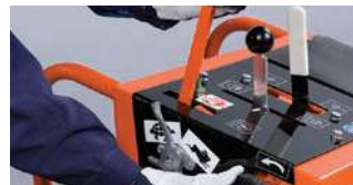
MANUAL OR HYDRAULIC RAISE & LOWER THE BLADE
