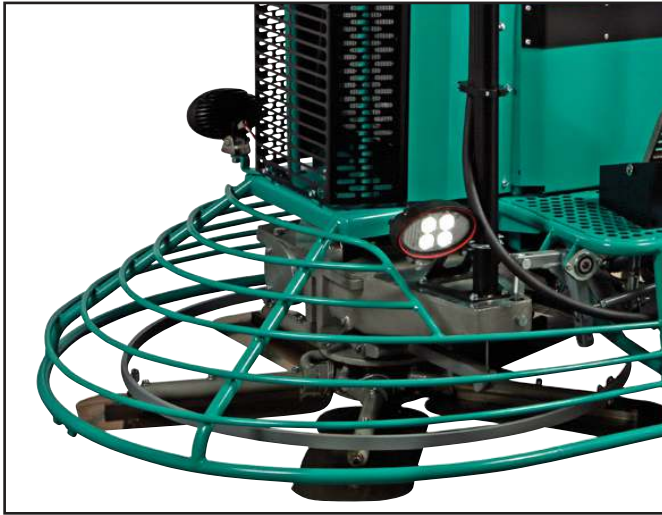
LED lighting provides state of the art illumination for night time or inside work
