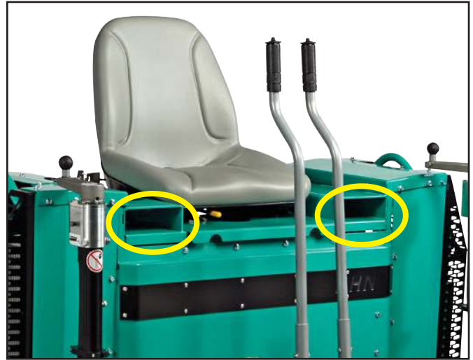
Fork truck pockets built into an ergonomically designed seat frame
